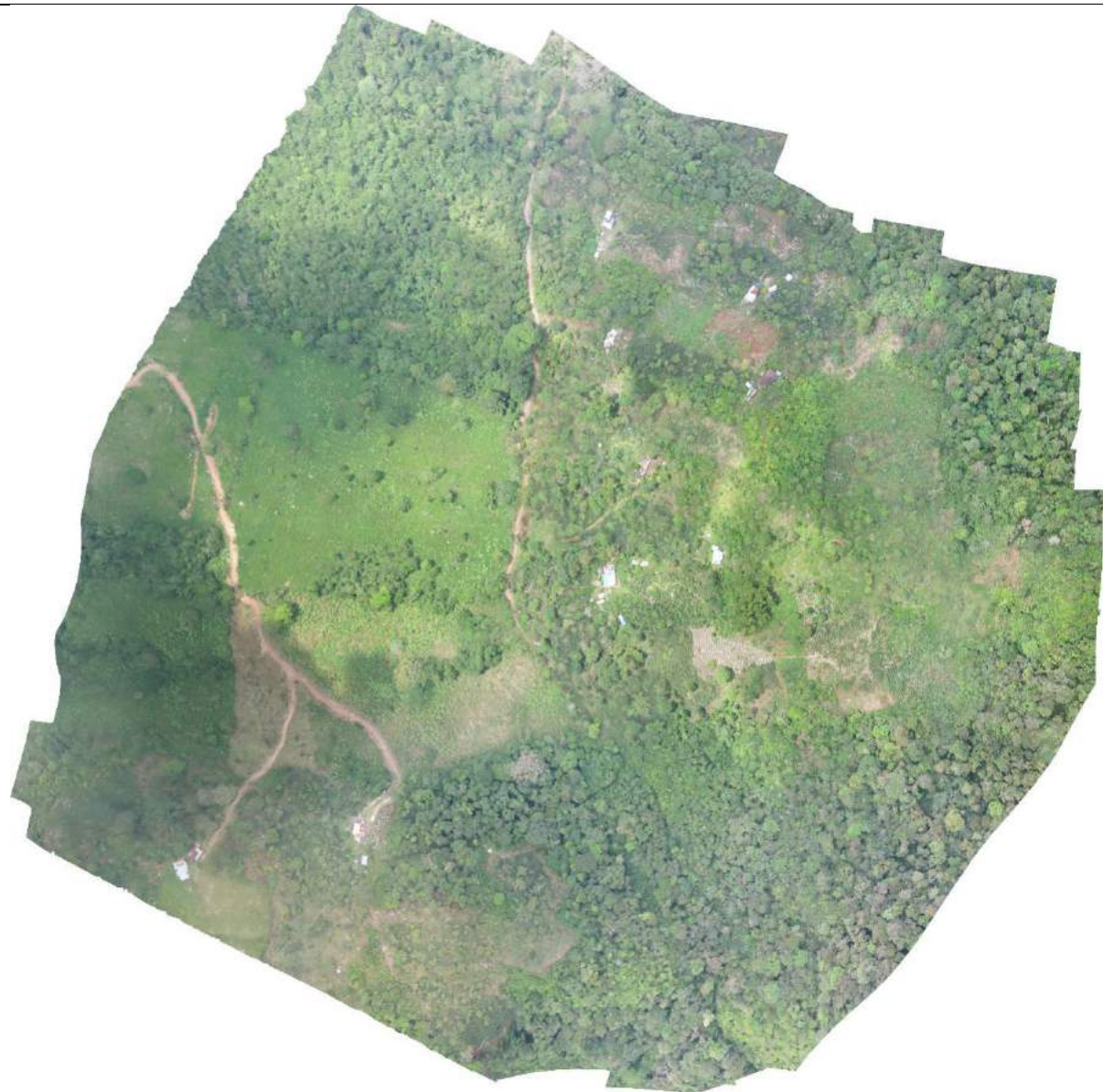
H3.13. Orthomosaic generated by AGISOFT PHOTOSCAN from aerial images taken by VANT. ©UIS/Sergio Bolívar & Mateo Jaimes
