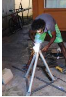
Creation of the tool for IAS roots removal @ EPCO/Estelle DEJA
