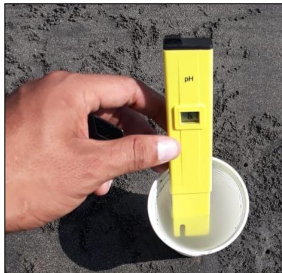
Photo 1. Sampling of parameters in water such as pH, dissolved oxygen, and temperature. Credits: Kevin Reyes, FIDES.
