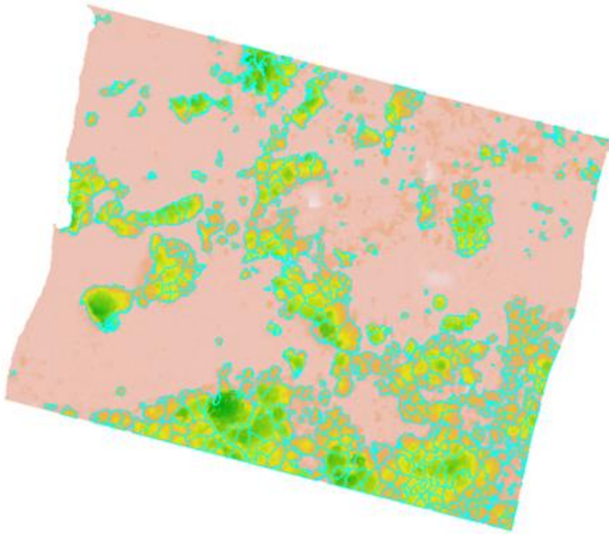
Picture H2f. Canopy height model with polygons to calculate the area of the canopy for each tree. Image generated by biology student, UIS ©Mateo Jaimes
